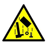
FALL OF THE LOAD OR OBJECTS FROM THE TOP. MAKE SURE OF THE LOAD STABILITY ON THE SHELF, USING, IF NECESSARY, SAFETY SLING ROPES.
