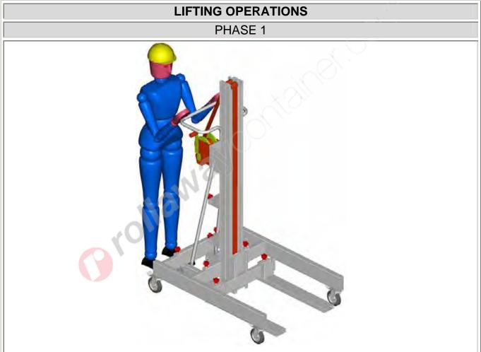
Place the hoister in the working area according to the CARRIAGE AND STORAGE INSTRUCTIONS.
